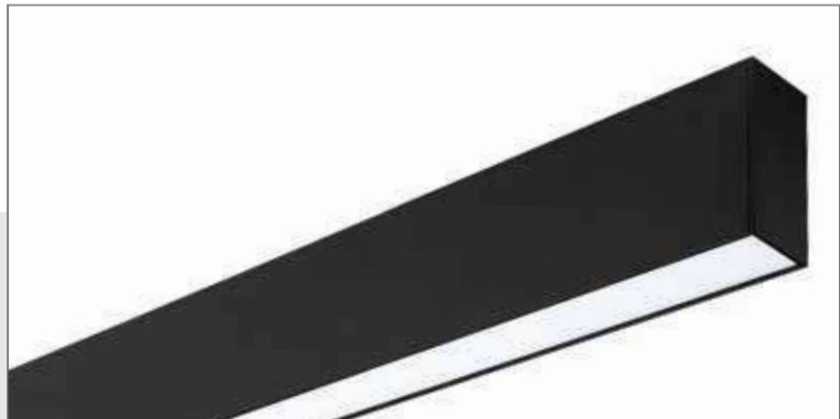
34mm LED profile luminaire, made of an extruded aluminium, power-coated with fine sandy finish. Designed for ceiling/pendant/trim-less/recessed mounting, providing direct light emission through PMMA diffuser. Luminaire equipped with the latest generation of well known LED boards with small color tolerance.
